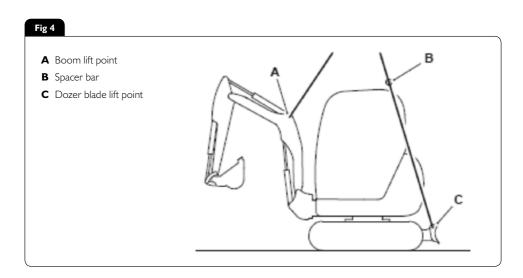
The correct lifting positions are identified on the machine by their labels:
