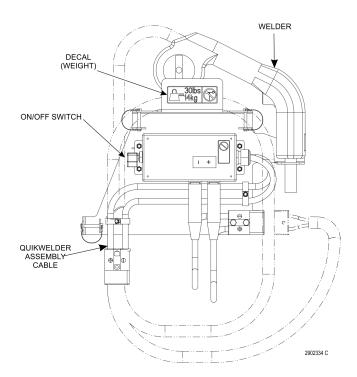
**NOTE:** QuikWelder can be installed simultaneously with either the Panel Carrier or Pipe Racks; however, the two accessories must be mounted on opposite sides of the platform.
