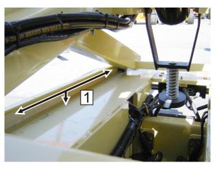
Figure 6-2. Lower Slide Pad Channel
