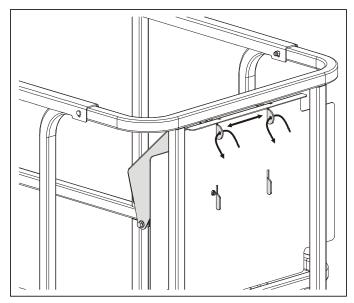
Figure 3-8. Securing Control Station to Platform
