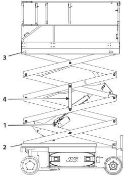
Figure 6-1. Lubrication Diagram
