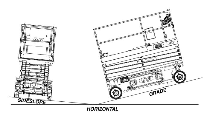
Figure 3-5. Grade and Sideslope - Driving - Platform Stowed
