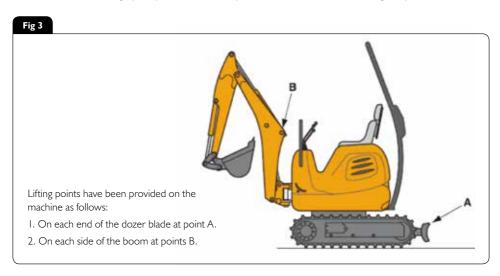
The correct lifting positions are identified on the machine by their labels:
