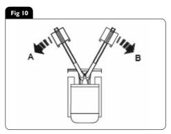
WARNING: The swing and auxiliary pedals must be in their folded positions when not in use.
